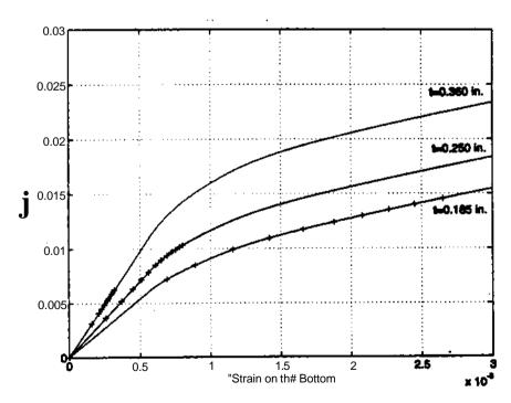
FIGURE 6: Plot Showing Values of £pe<sub>en</sub> Predicted by the Beam-Based Analysis with the Strains Measured After Each Pass of Peening
