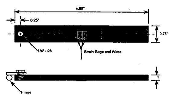
FIGURE 1: Diagram of the Specimens Used in the Free Peening Tests
