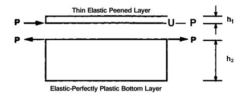
FIGURE 3: Decomposition of the Specimen into Two Beams
