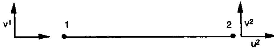
**Figure 5:** Displacements at the nodes of a truss element
