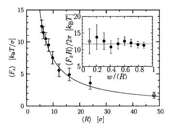
FIG. 4. Tensile force  $\langle F_z \rangle$  as a function of cylinder radius  $\langle R \rangle$  for the systems with N=5000 lipids (with the exception of the open symbol, which has  $N=10\,000$  lipids). The solid line is a fit to Eq. (7), leading to  $\kappa=11.7k_BT$ . The inset shows the combination  $F_zR/2\pi$  as a function of rescaled curvature  $w/\langle R \rangle$ , and the solid line again indicates  $\kappa=11.7k_BT$ .
