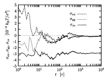
FIG. 3. Running average of the diagonal components  $\sigma_{xx}$ ,  $\sigma_{yy}$ , and  $\sigma_{zz}$  of the stress tensor for a cylindrical vesicle with  $\langle R \rangle = 70\sigma$ .
