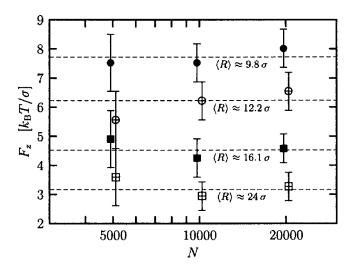
FIG. 5. Tensile force  $F_z$  as a function of system size for systems of different ratio  $L_z/N$ : ( $\bullet$ ) 0.01, ( $\bigcirc$ ) 0.008, ( $\blacksquare$ ) 0.006, and ( $\square$ ) 0.004. The corresponding average radius  $\langle R \rangle$  is also indicated. A slight horizontal offset is included to improve visibility of the error bars.
