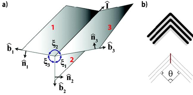
FIG. 1 (color online). (a) Illustration of triple-junction geometry.  $\xi_i$  denotes the dihedral angles,  $\mathbf{l}$  the triple-junction line,  $\mathbf{b}$  is the boundary tangent, and  $\mathbf{n}$  is the boundary normal. (b) Illustration of symmetric tilt grain boundary in lamellar system. The boundary (indicated as bold) bisects the tilt angle  $\theta$ .
