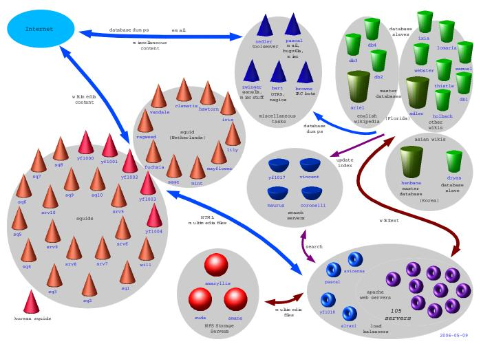
Figure 1. The Wikipedia infrastructure in May 2006 (from <a href="http://en.wikipedia.org/wiki/Wikipedia">http://en.wikipedia.org/wiki/Wikipedia</a>). In May 2007 the infrastructure has a similar architecture, but the number of servers has increased by 64% to sustain a 100% increase in the incoming load.
