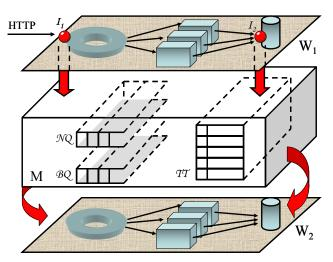
Figure 4. Dependency-agnostic upgrades. The old and new versions are installed and execute in parallel universes  $W_1$  and  $W_2$ . MetaMorphMagi intercepts the request flow at the ingress ( $I_1$ ) and egress ( $I_2$ ) points of the old version. The rest of  $W_1$  is treated as a black box.
