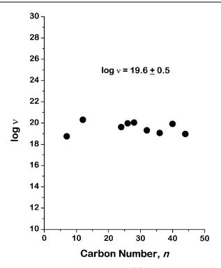
FIG. 2. The preexponential factors  $(\nu)$  of the first-order desorption rate constants (k) for alkanes of varying chain length (n=7 to 44). These were determined from thermal desorption spectra obtained at varying heating rates  $(\beta=0.1 \text{ to } 5 \text{ K/sec})$ . The value of  $\log(\nu)$  is apparently independent of alkane chain length.
