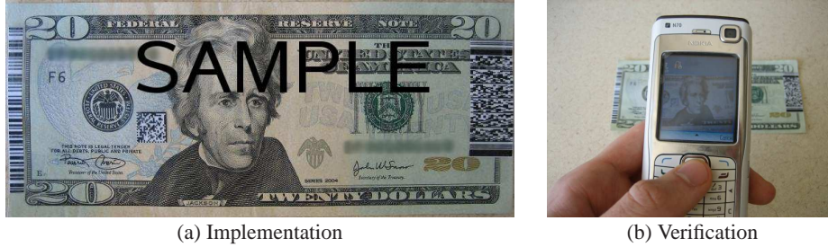
Figure 1: Barcode Signatures. A sample implementation of physical digital cash using 2-D barcodes to encode a signature of authentication. Anyone with an appropriate scanner or camera phone can verify that a legitimate institution issued this bill (or one identical to it).
