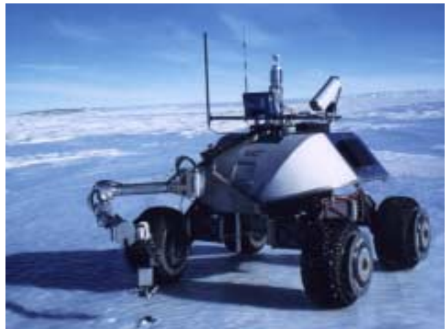
Figure 1: Nomad investigating a meteorite sample using its manipulator arm at Elephant Moraine, Antarctica.
