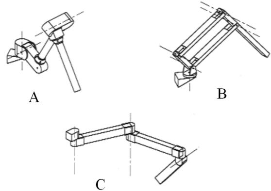
Figure 2: The revolute (A), 5-bar (B) and SCARA concepts (C).
