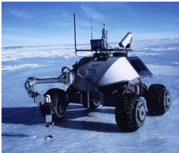
Figure 8: Nomad with the sensor arm deployed.
