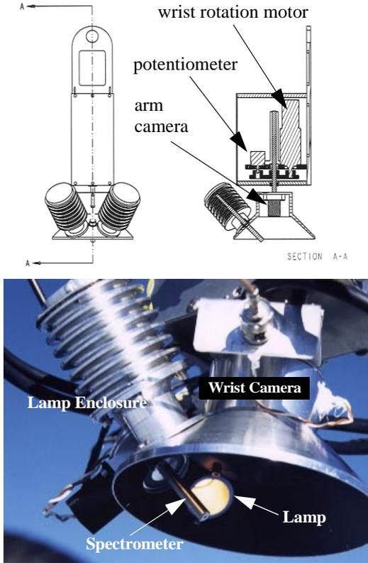
Figure 3: The sensor head.
