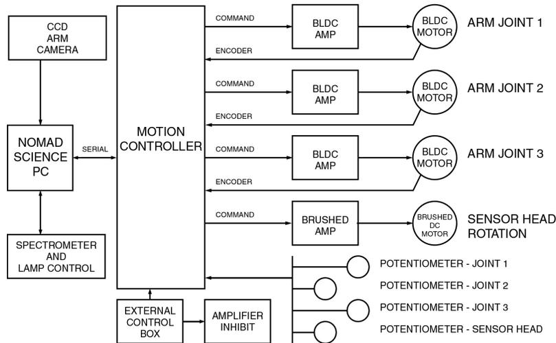
Figure 7: Block diagram of the sensor arm electronics.
