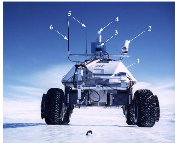
Figure 1: Nomad components: (1) sensor arm (shown stowed), (2) high-resolution science camera, (3) laser range finder, (4) panoramic camera, (5) radio modem antenna, (6) high-gain wireless ethernet antenna.
