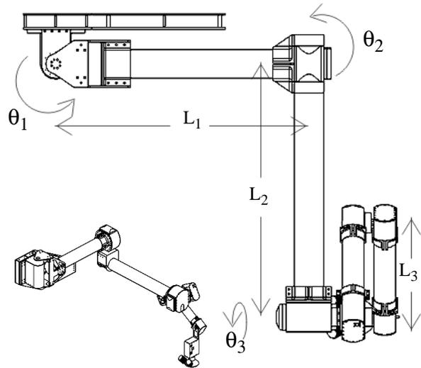
Figure 4: Sensor arm schematics
