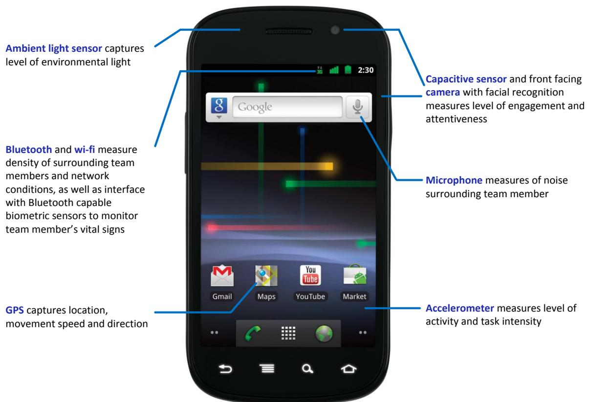
**Figure 2. Sensors on a Google Nexus S mobile device**
