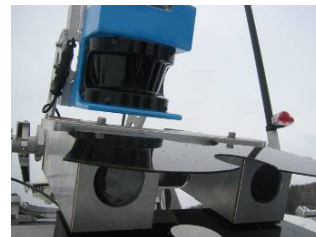
Figure 4 Nomad is equipped with binocular stereo cameras, in sealed, heated enclosures, for dense range information in the near field. A single-axis, scanned laser rangefinder also swept a single line across the path to detect obstacles.
