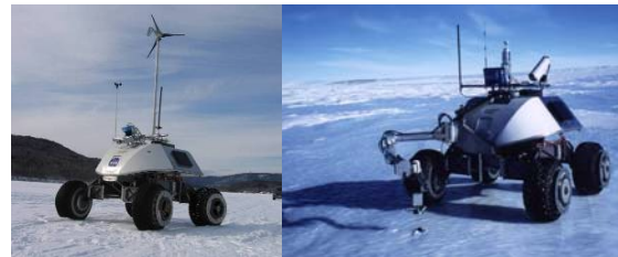
Figure 2. LORAX robotic rover (Nomad) undergoing tests on frozen lake Mascoma, New Hampshire (February 2005), and searching for meteorites in Antarctica (January 2000)
