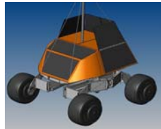
Figure 9 Nomad solar panel configuration
