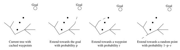
Fig. 4. Extended RRT with a waypoint cache for efficient replanning.
