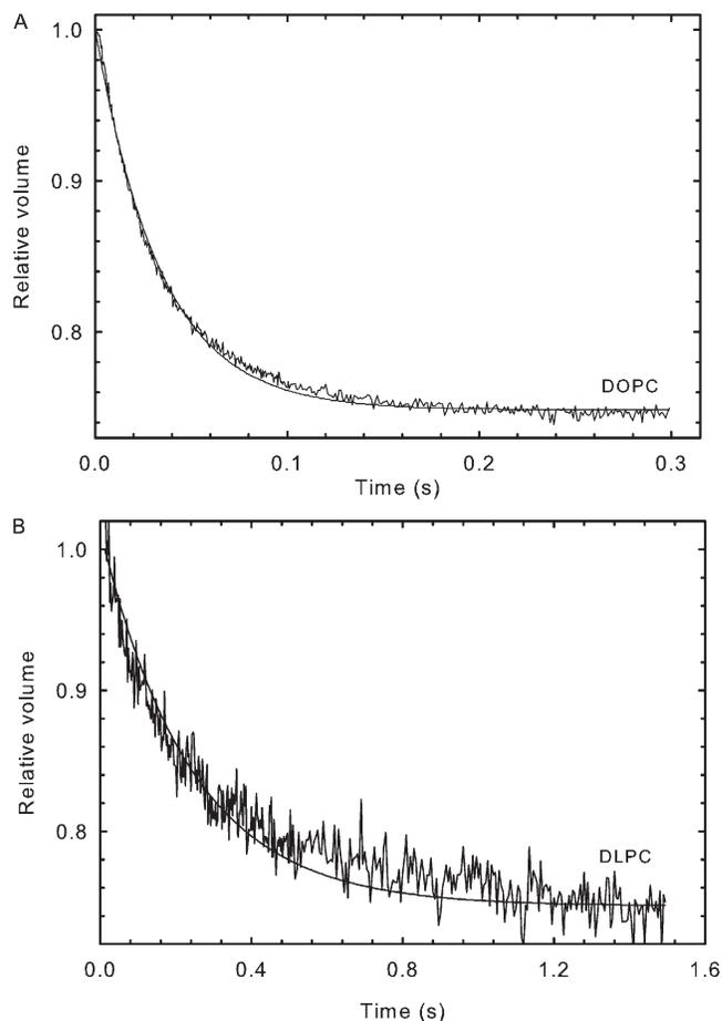
**Figure 1.** Water permeability measurement. Time trace of volume change of liposome measured by fluorescence quenching, DOPC (A), or light scattering, DLPC (B). Liposomes were subjected to a 50% increase in external osmotic pressure.
